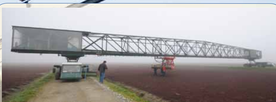
This is mechanisation! The machine strips surplus growth from the cranberry bogs. Powered by a tractor engine in each 'pod', it was built entirely in Cran Chile's on-site workshops. Seats courtesy of an old Opel Vectra.
